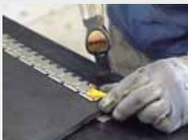
1) Square the belt end and place the fastener adapting it to the thickness of the belt; apply the pins to the head on a metal plate
