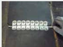
5) Repeat on the second belt end, place it over the first and insert the fixing wire
