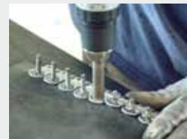
2) Insert the bolts and tighten them with the nut tightener
