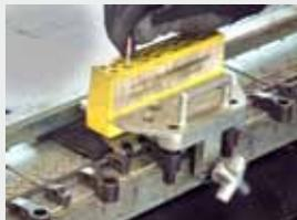
2) Position the rivet applicator and insert the rivets
